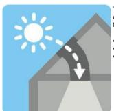
The **flexible** tunnel is ideal for distances between roof and ceiling from 0.4 to 1.5 m.
